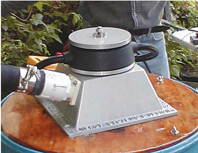
A Canadian-made Energy Systems and Design turbine uses a permanent magnet alternator and a turgo runner.
