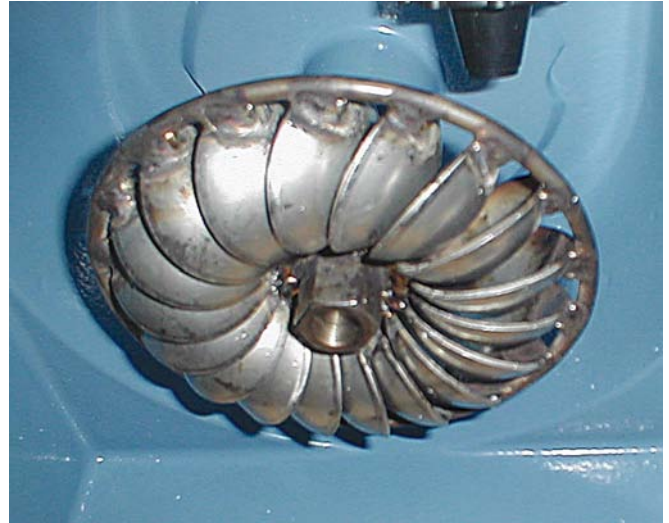
Shown from beneath—the 4-inch (10 cm) turgo runner in an Australian-made Platypus turbine.
