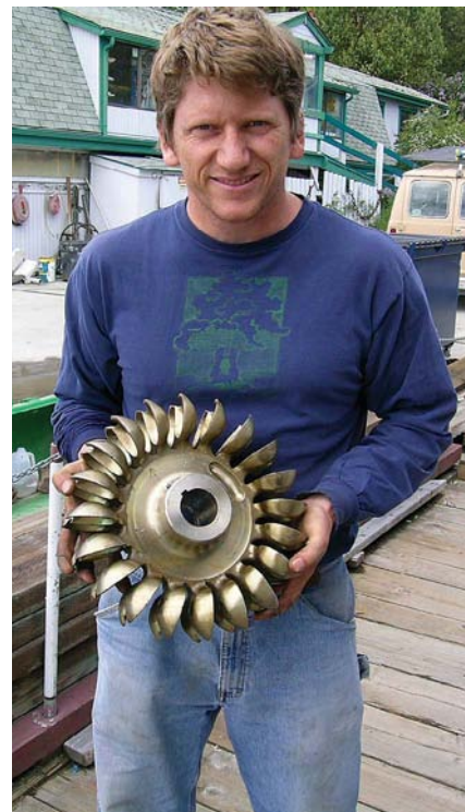
The author with the 10.5-inch Pelton runner for the Canyon Industries turbine.
