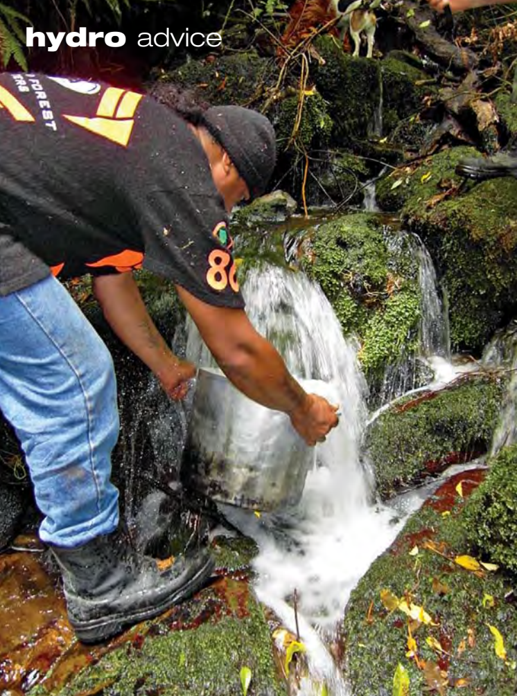
The “bucket method” can be used to measure flow in small streams. Larger streams require an alternative measurement method.
