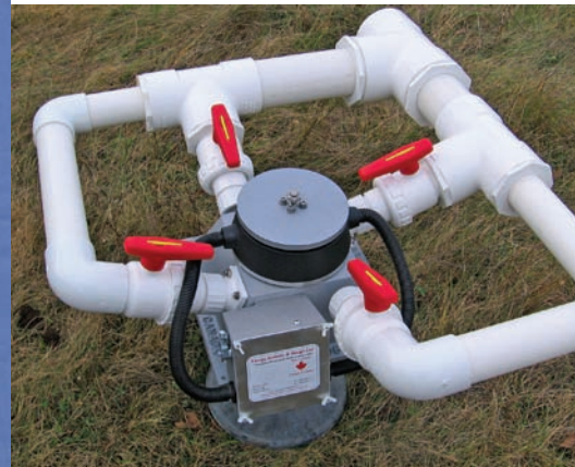
Energy Systems & Design turgo turbines use permanent-magnet alternators to produce up to 1 KW at 12 to 240 VDC.
