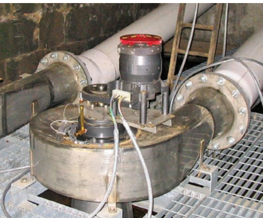
The Nautilus Francis-style turbine is designed for low-head applications and produces up to 3.4 KW. It can be used with a variety of generators and voltages.
