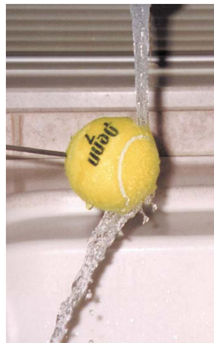
The Coanda effect is demonstrated by the water adhering to the surface of the tennis ball.
