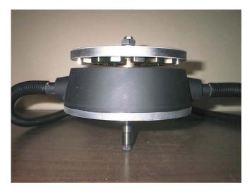
Like this Energy Systems & Design alternator from a Stream Engine turbine, many small, DC, hydroelectric units now use more efficient, brushless, permanent magnet alternators.
