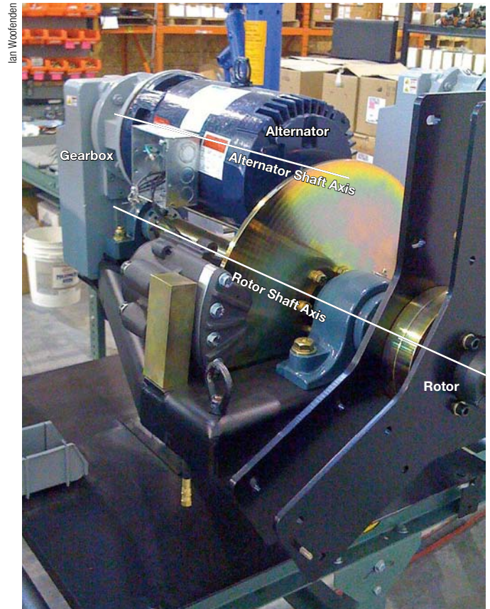
In some cases, a gearbox is necessary to optimize blade/rotor rpm with alternator rpm (also note this turbine's large disk brake).
