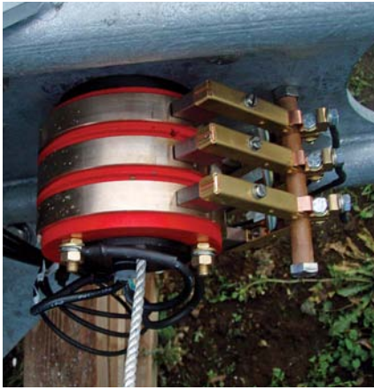
Brushes transmit electricity from a yawing turbine down a stationary tower without twisting wires.
