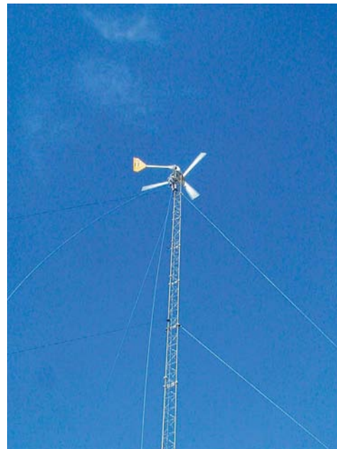
Right: A side-furling governor uses the force of the wind on an off-center joint to pivot the blades out of the wind. In this case, mechanical furling is used to brake the machine during maintenance.
