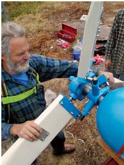
Left: Centrifugal force on the blades works a linkage to change blade pitch on an old Jacobs generator. This complex but highly effective governor precisely regulates rpm.
