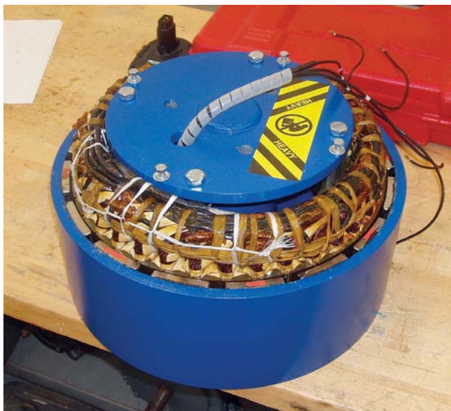
Permanent magnets on the outer rotor allow a simple brushless design. The windings are mounted on the inner immobile stator.
