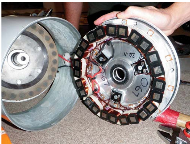
This axial PM alternator has magnets on its rotor that spin past stationary coils face to face.
