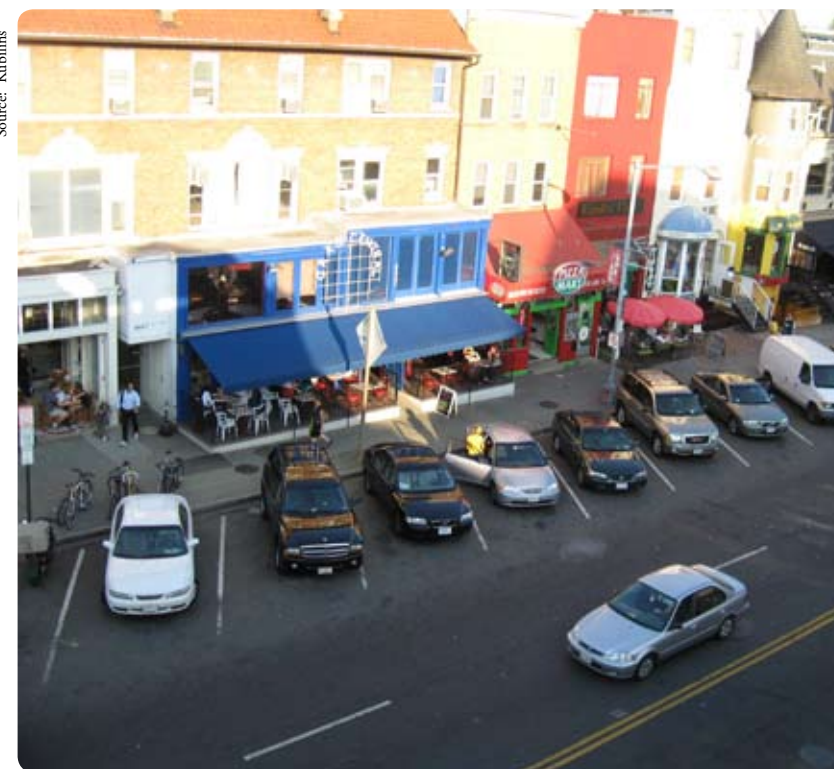
An example of back-in angle parking on the main commercial street in the Adams-Morgan district of Washington, DC.
