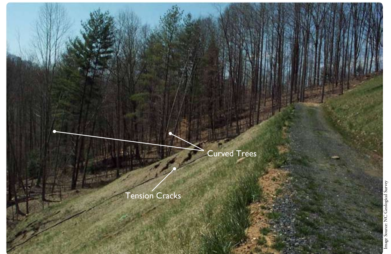
Tension cracks and curved trees, both indications of slope instability, can be seen in this photo from western North Carolina.
